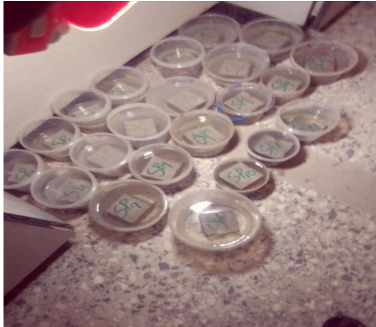
Plate 1: Cement sheath system cured for 7 hours.
