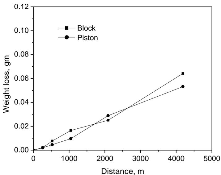
**Figure 1.** Variation of Weight Loss (gm) with the Variation of Sliding Distance (m) at Applied Pressure of 1.4 MPa (Load = 20 N) and Sliding Velocity 0.29 ms<sup>-1</sup> in Dry Condition.
