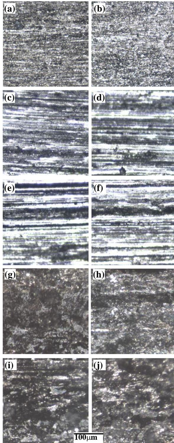
**Figure 5.** Optical Micrograph of Worn Surfaces before Wear a) Block, b) Piston, after Wear at Applied Pressure of 1.40 MPa for 15 min c) Block, d) Piston, for 4 hr e) Block, f) Piston, Corrosive Environment at Applied Pressure of 1.40 MPa for 15 min g) Block, h) Piston and for 4 hr i) Block, j) Piston.
