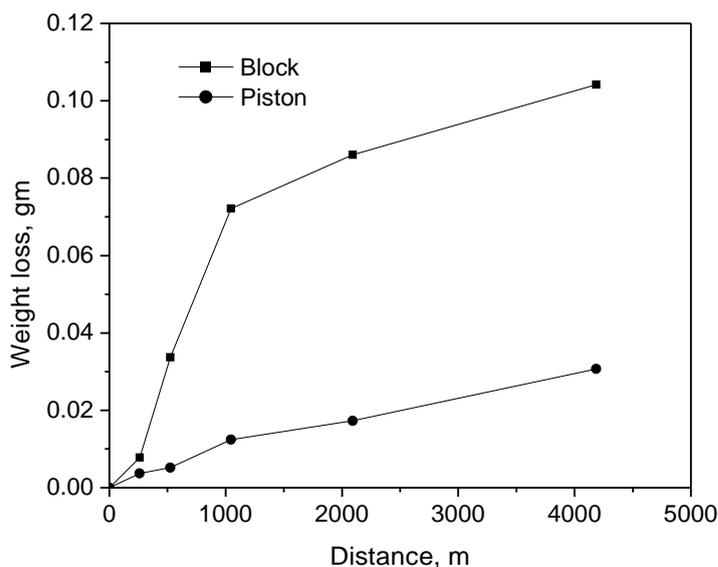
**Figure 2.** Variation of Weight Loss (gm) with the Variation of Sliding Distance (m) at Applied Pressure of 1.4 MPa (Load = 20 N) and Sliding Velocity 0.29 ms<sup>-1</sup> in Corrosive Environment.
