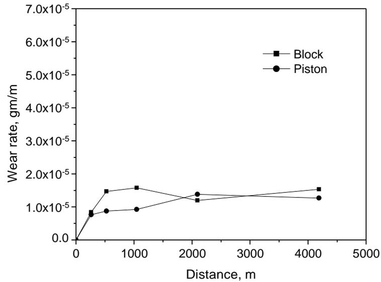
**Figure 3.** Variation of Wear Rate (gm/m) with the Variation of Sliding Distance (m) at Applied Pressure of 1.4 MPa (Load = 20 N) and Sliding Velocity 0.29 ms<sup>-1</sup> in Dry Condition.
