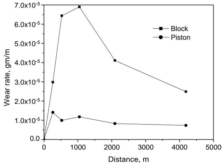
**Figure 4.** Variation of Wear Rate (gm/m) with the Variation of Sliding Distance (m) at Applied Pressure of 1.4 MPa (Load = 20 N) and Sliding Velocity 0.29 ms<sup>-1</sup> in Corrosive Environment.
